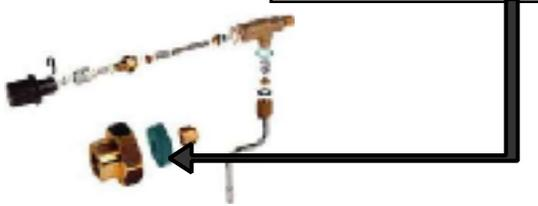
In order to grant a better sealing of the above mentioned gasket and optimise its working condition with regards to the new steam valve, we inform you that from the month of September the gasket will be softer than the former ones. The part number will not change
